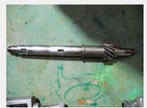
• Bristol 400 Gearbox layshaft reconditioned by Bristol Cars UK.
