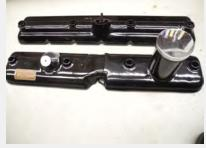
• Bristol Engine Set of RH & LH Rocker covers two pack painted, LH rear rocker cover with oil filler spout.
