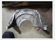
Bristol 6 cyl engine lower cast flywheel cover.
