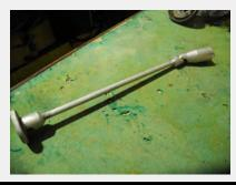
Bristol Original Plug Spanner Part No N600010 with insert to suit 10mm current Bristol spark plug. Rare
